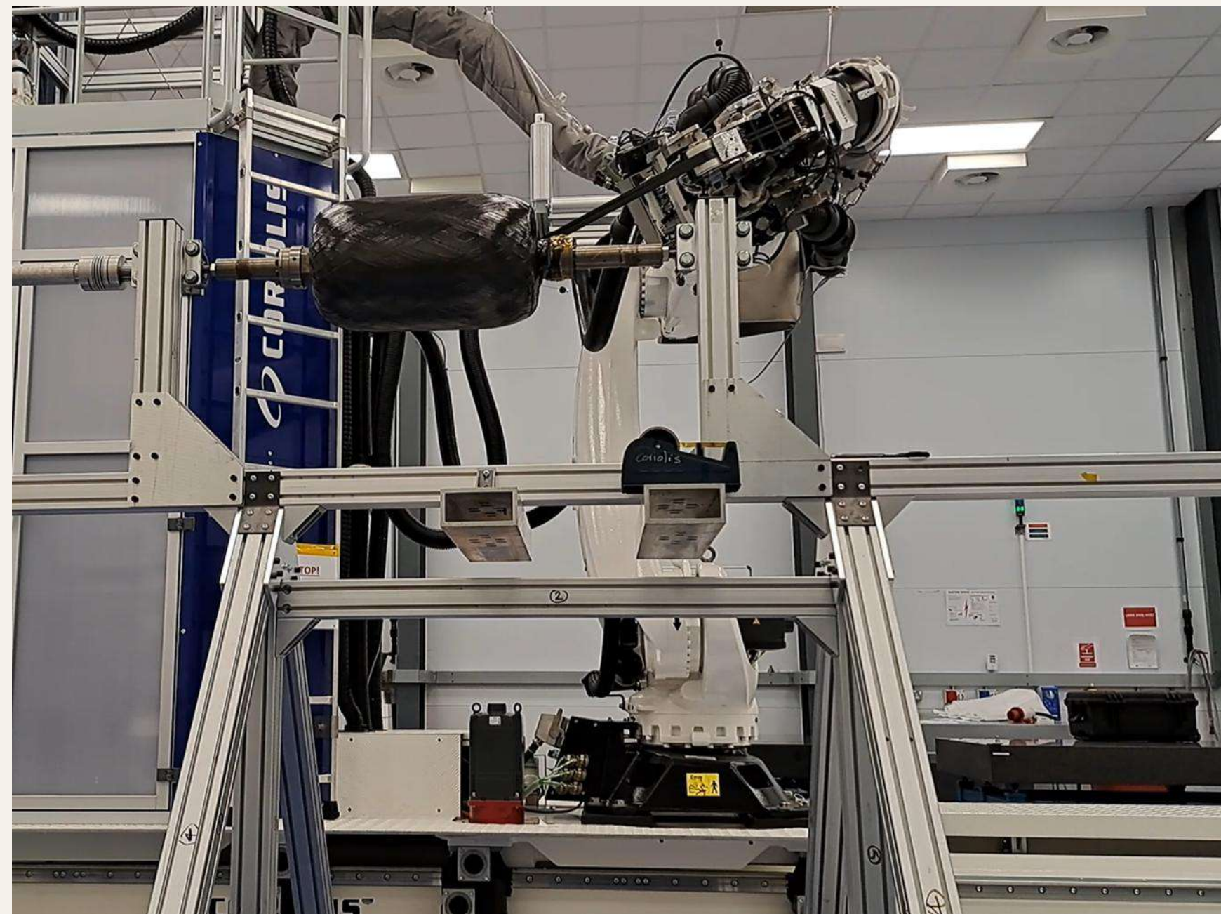
Composite wrapping process using Automated-Fiber-Placement
