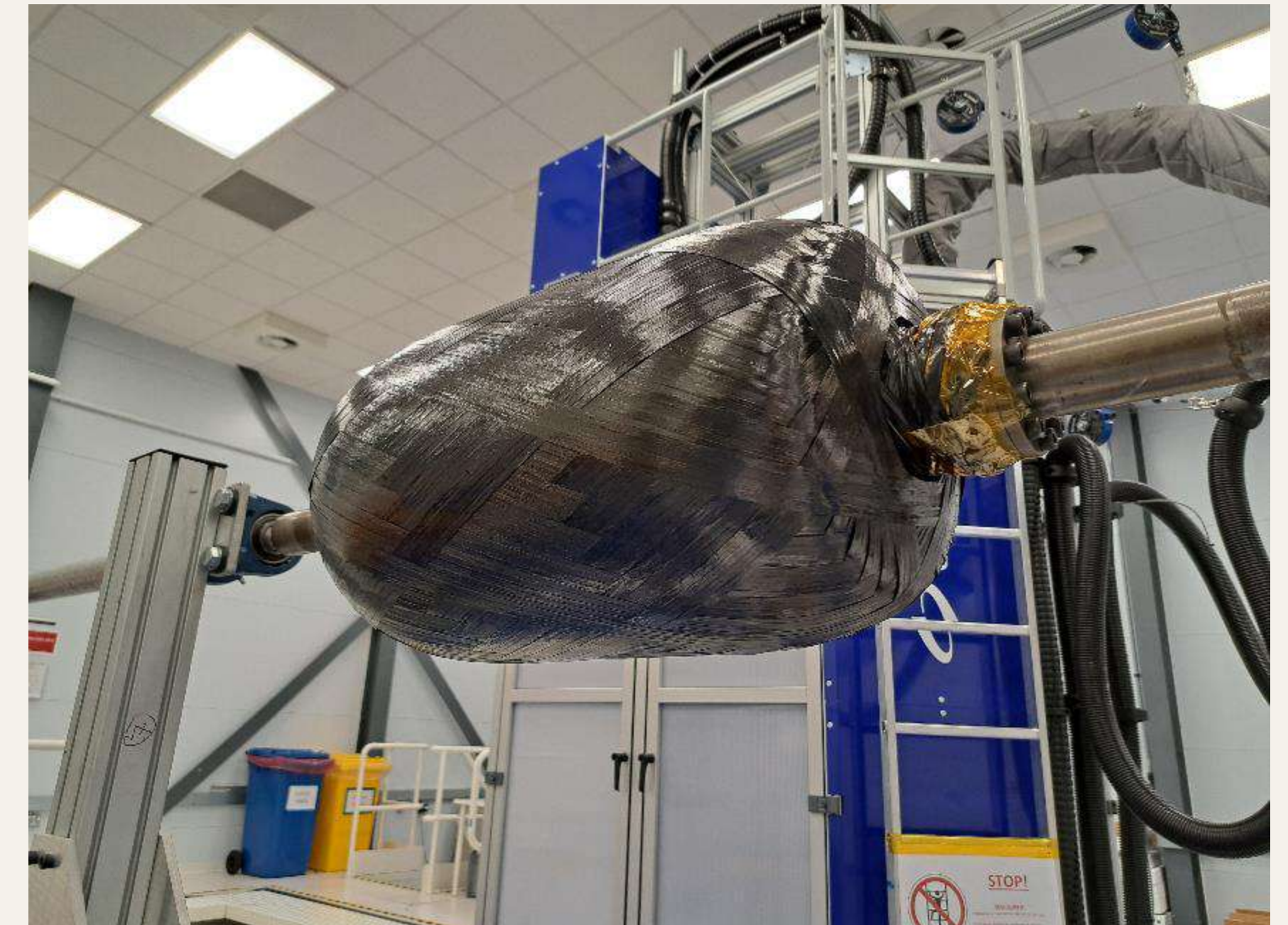
Wrapped composite tank ready for curing step in autoclave
